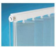
Vertical blinds should be manufactured using the Slimline headrail system with aluminium headrail of 29.25mm (15/32") width and 27.75mm (13/32") depth.
